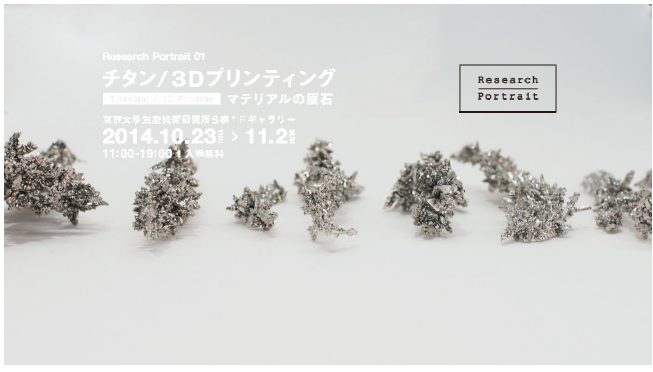
Fig. 4 Dendritic titanium crystals produced by molten salt electrolysis are displayed as design/artistic products. ( http://www.design-lab.iis.u-tokyo.ac.jp/exhibition/rp01/ )
