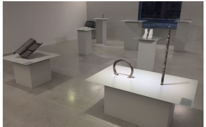
Fig. 3 Titanium cover plate for use in roof of temples (left in the photo), ultra-high purity titanium crystal bar and tubes are displayed as design/artistic products (right in the photo).
